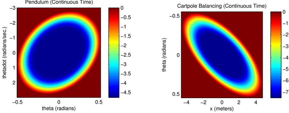
Figure 3: The log-base-10 failure probabilities for two continuous-time systems. Left: balancing for the pendulum, as a function of initial conditions. Right: balancing for the cartpole, as a function of initial conditions in  $x$  and  $\theta$  (the initial conditions for  $\dot{x}$  and  $\dot{\theta}$  are fixed to 0).
