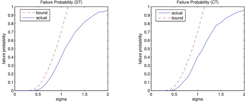
Figure 1: True probability of failure (blue) versus computed probability bound (red) as a function of the noise variance. Left: discrete-time. Right: continuous-time.
