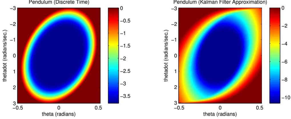
Figure 2: The log-base-10 of the failure probability for the discrete-time pendulum after one hour. Left: failure probability plotted against initial conditions, verified with our algorithm. Right: estimated failure probability for the linearized discrete-time pendulum, computed with a Kalman filter.
