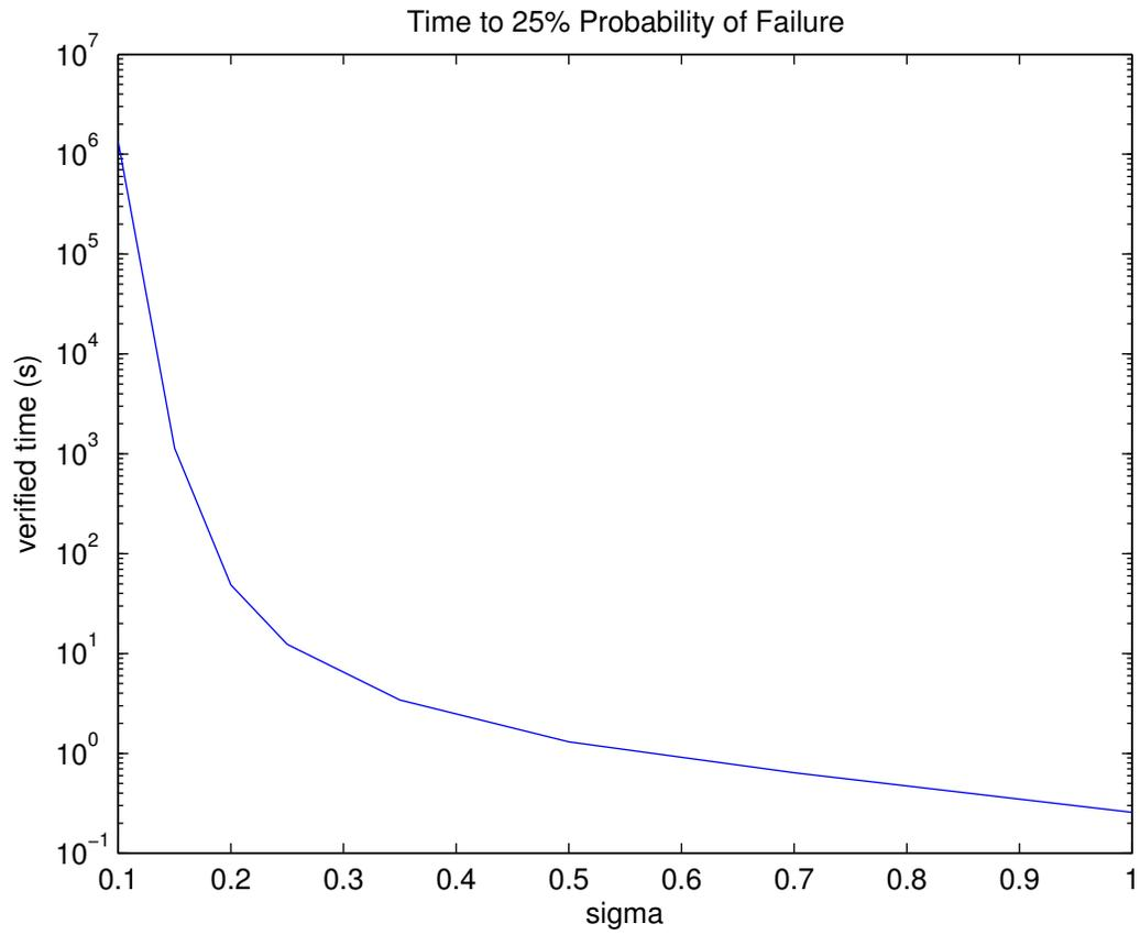
Figure 4: Verified time to failure versus  $\sigma$  (turbulence intensity) for the quadrotor.
